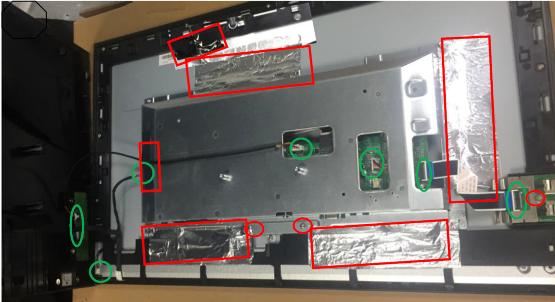
S7. Prepare a rear cover to assemble it. Use the screws to lock the rear cover.
