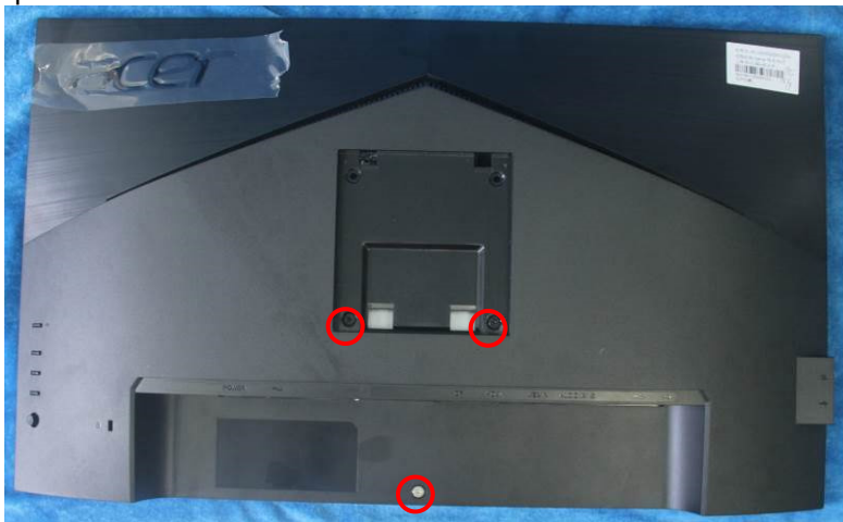
S8. Assemble the stand ASS'Y to rear cover.
